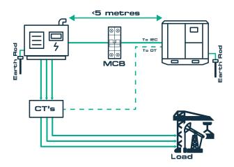
Peak Power 200 reacts to frequency voltage and power changes on the microgrid between power source and application. The Peak Power 200 can be used alongside a diesel generator or it can be connected to the grid / battery.
