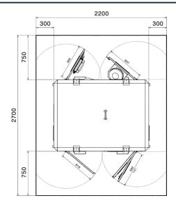
Dumarey Flybrid recommend a space of 2700mm x 2200mm be left around the unit. This is to ensure that there is enough space to open the front and rear service doors to enable maintenance of the unit.
